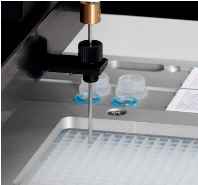
Dissolved peptide-cellulose conjugates in 384 well being spotted onto CelluSpots slides.
